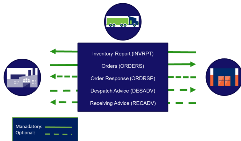
Figure 30: EDI Communication Process (Source: GS1)
